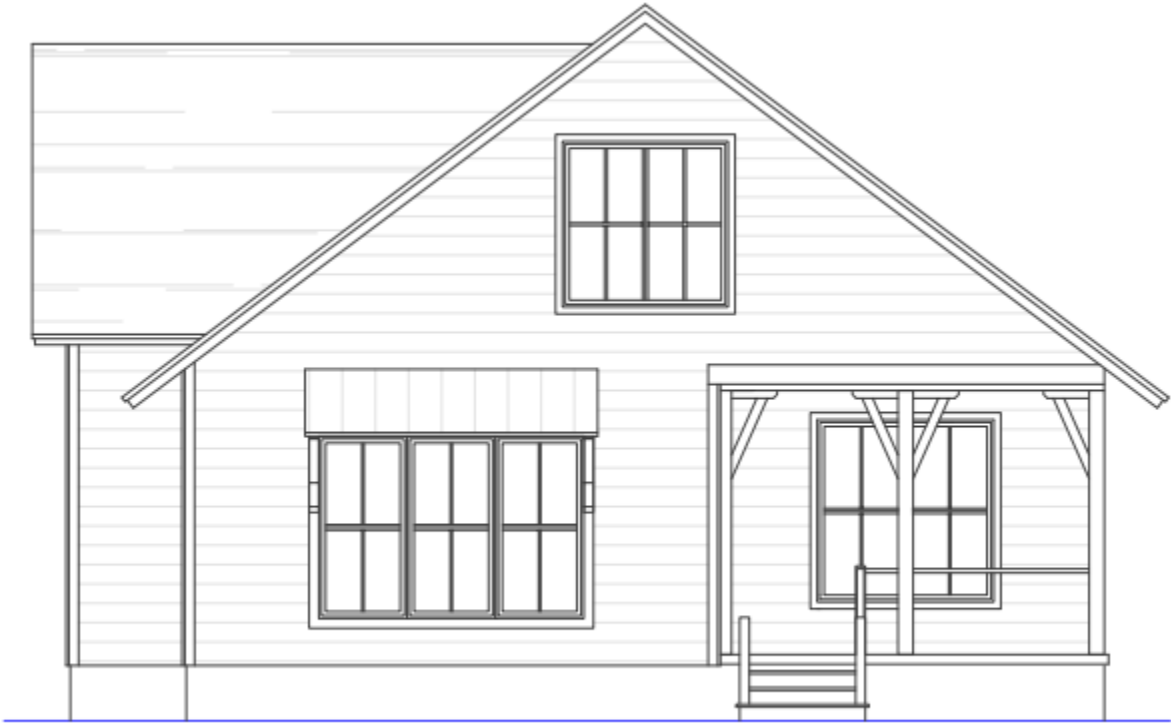
Front Elevation - 8' ceiling height
